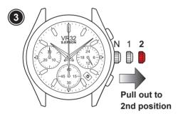
• Pull the crown out to the 2nd click position when the second hand is at the 12 o'clock position.
